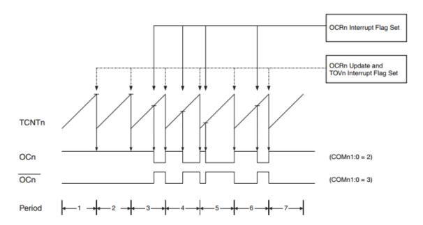
In the above picture, Compare Output mode (COMx1:0) is set in such a way that the OCx gets set whenever an overflow occurs, and to clear the OCx pin whenever an output compare match occurs (i.e. COMx1:0=2). The same timing diagram in the case of Timer 1 is shown below. Please note that the OCn and its compliment shown in the figure below are wrong. You can see that in the case of Timer/Counter 1, the value till which TCNTx counts is determined by the TOP value.
