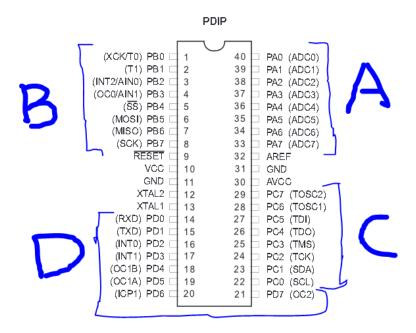
It is clear that the each of these ports contain 8 pins each. For example, PORTA contains pins PA0...PA7. They are clubbed into 8 because the microcontroller is 8-bit. Each port is byte addressable. We will come to that later. So in total there are 32 GPIO pins in an ATmega 16.
