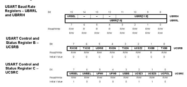
The above figure shows the three registers that need to be configured to properly initialize the UART module.
