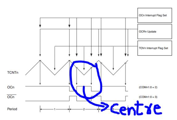
From the timing diagram, it is evident that the TOP value is constant and equal to MAX in the case of Timer/Counter 0 and 2. The following is the timing diagram in the case of Timer/Counter 1. It should be noted that the TOP value in
