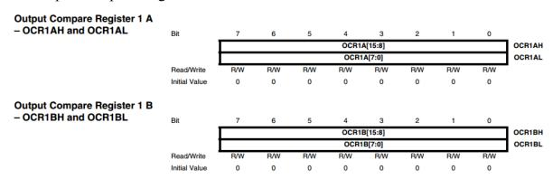
As explained earlier, the OCR1A and OCR1B are capable of making two independent square waves on the OC1A and OC1B respectively.
