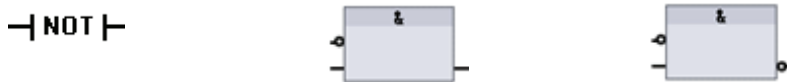
LAD: NOT contact inverter FBD: AND box with one inverted logic input FBD: AND box with inverted logic input and output
