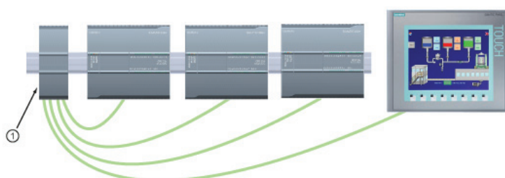
Network connection: More than two devices connected together, using a CSM1277 Ethernet switch ①
